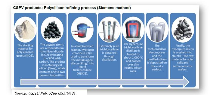
The USITC described the Siemens and fluidized bed reactor processes in narrative as
