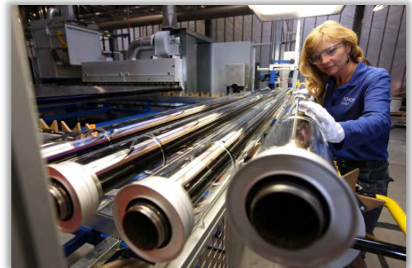
Worker inspects CSP receiver tubes at SCHOTT Solar in Albuquerque, NM. (SCHOTT Solar)
